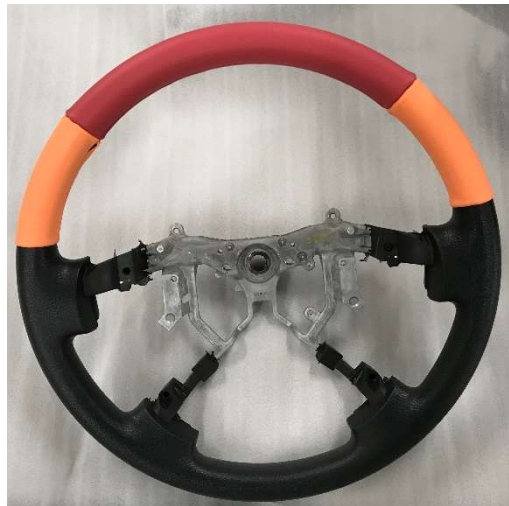
Figure 7. Prototype of a colored fluoroelastomer steering wheel cover (the orange and red parts are made of fluoroelastomers)
